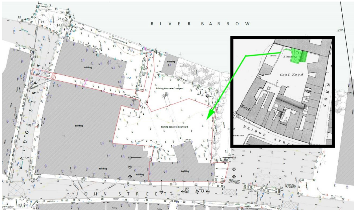
Fig.23: The concrete ground surfaces at courtyard level within the red line are to be removed to a depth of 500mm; the area may retain traces of a lime kiln known from 19 th century maps (inset map shows the lime kiln as depicted on the 1881 OS map) as well as other below-ground archaeology.
