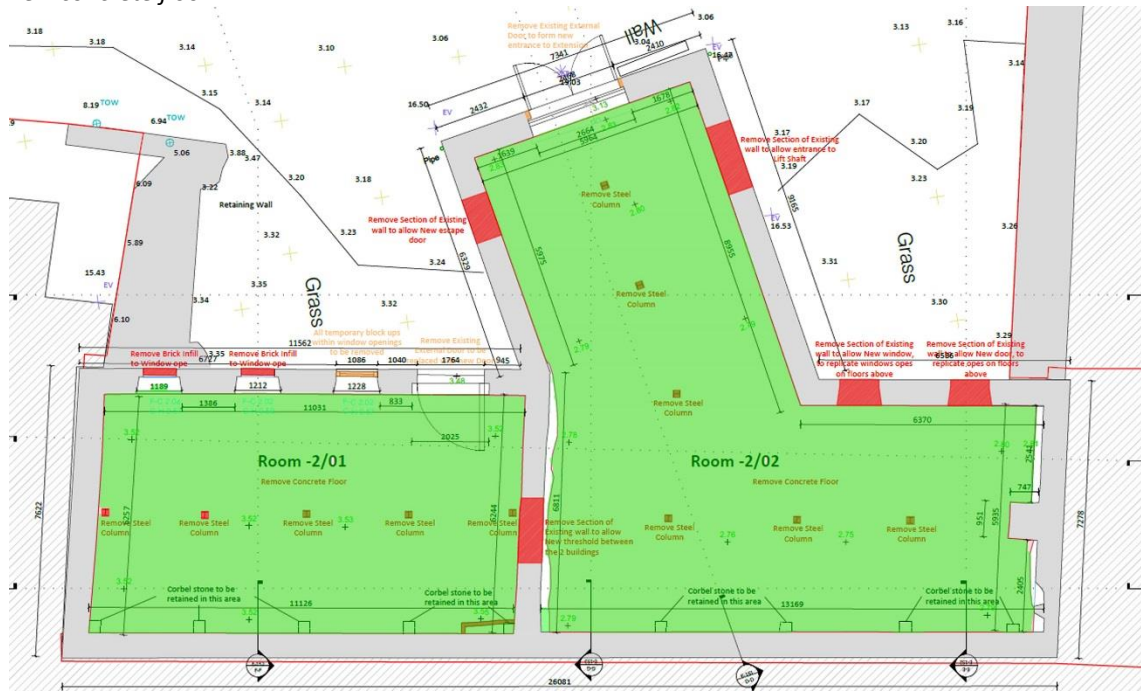
Fig.22: Plan view of the courtyard level (Level -2 on the ODKM drawings) showing the proposed removal of the existing concrete floor (highlighted in green) to a depth of c.500mm, and the removal of eleven (11 no.) steel posts.
